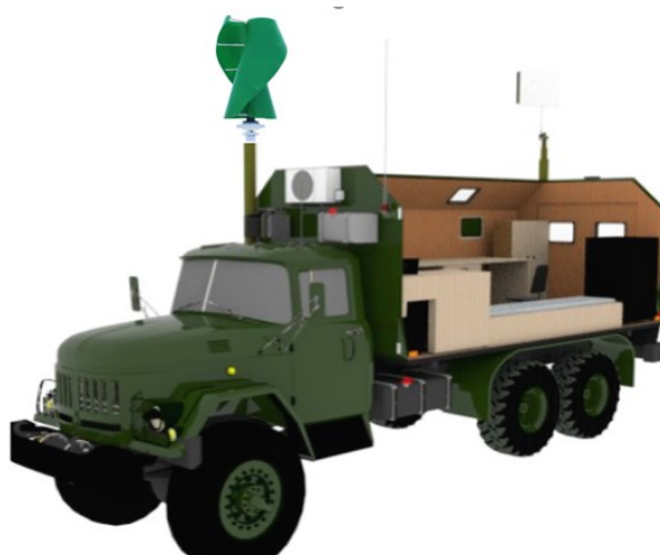
5-rasm. Universal aloqa majmuasiga shamol turbinasini o'rnatish chizmasi.
